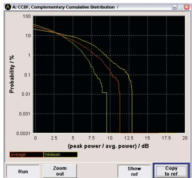
FIG 3 The built-in transients recorder can sample the baseband signals of the R&S®SMJ100A in realtime and offers various representations such as I/Q diagram, CCDF and constellation diagram (see below).
