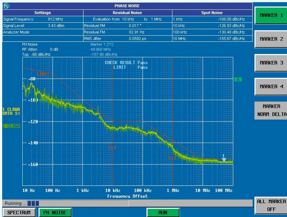
FIG 4 Typical result of a phase noise measurement at 10 Hz to 100 MHz offset from the carrier. The vertical red lines EL1 and EL2 mark the range limits for residual FM and \phi M measurements. The red curve is the user-defined LIMIT. The measurement result (Pass in this example) is displayed at the top center of the diagram. A smoothed trace (yellow) is superimposed on the original trace (green). The blue bar (Running) at the lower edge of the screen indicates measurement progress and helps you to assess the remaining measurement time.
