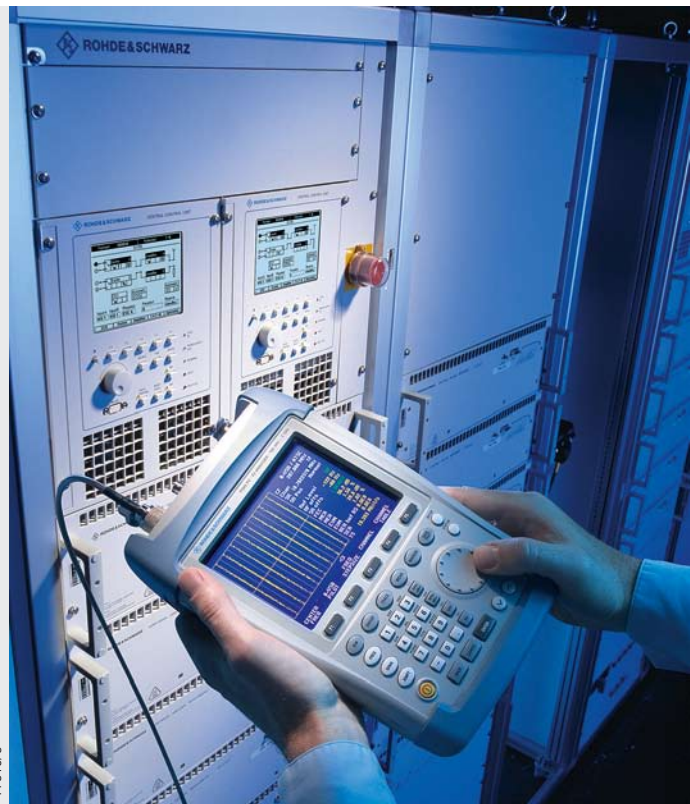
FIG 1 The TV Analyzer R&S®FSH3-TV was presented at NAB 2005 where it received three awards. The reason is clear: The innovative instrument can handle a wide variety of applications in the installation, maintenance and servicing of TV transmitters and cable networks.
