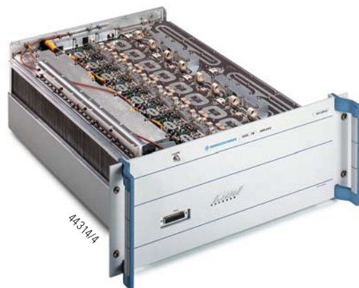
FIG 2 The R&S VU825 is modular in design and includes four identical 700 W base modules that are controlled by a 64 W preamplifier.
