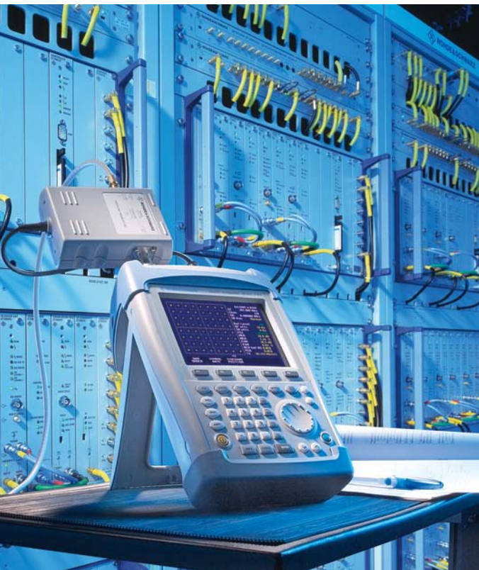
FIG 1 The TV Analyzer R&S®FSH3-TV was presented at NAB 2005 where it received three awards. The reason is clear: The innovative instrument can handle a wide variety of applications in the installation, maintenance and servicing of TV transmitters and cable networks.
